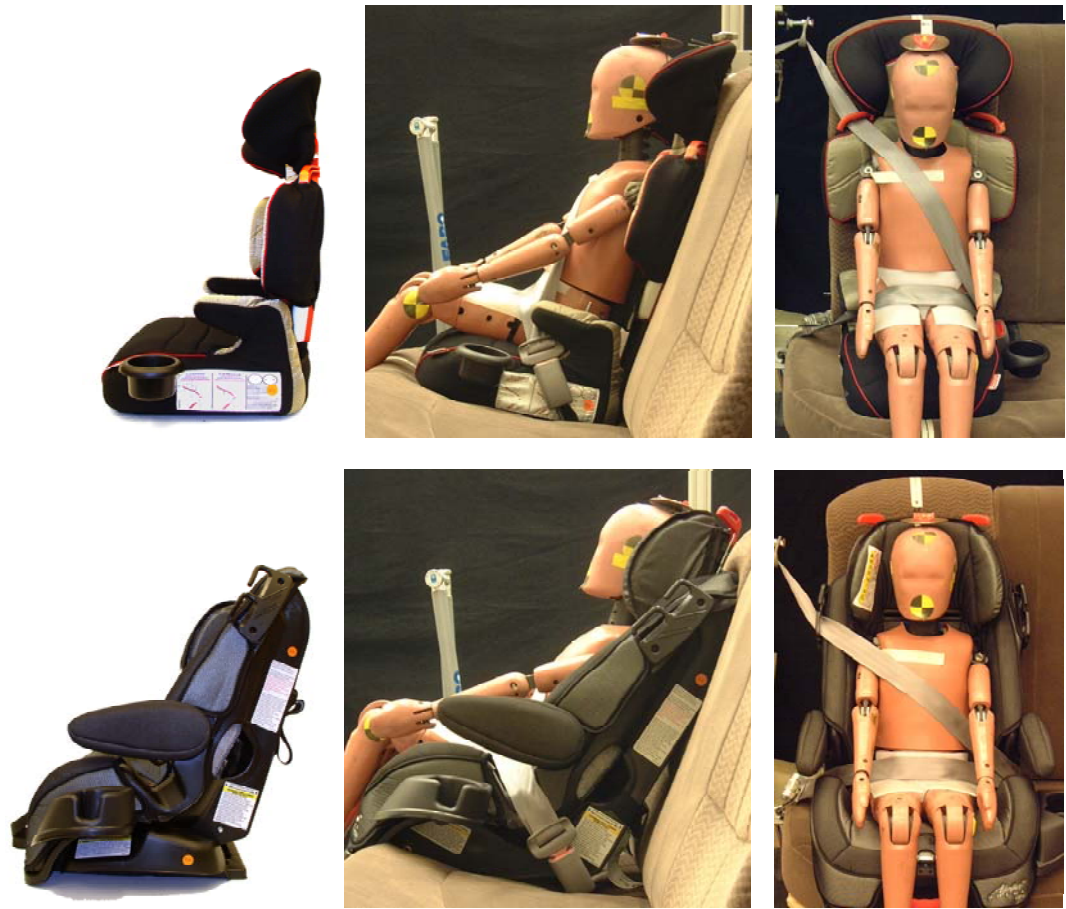
Figure 10. Design differences in lap belt routing features. Booster B19 (top) produced good lap and shoulder belt fit, whereas booster B24 (bottom) placed lap belt too high and shoulder belt too far outboard. Note placement of lap belt relative to ATD pelvis.
